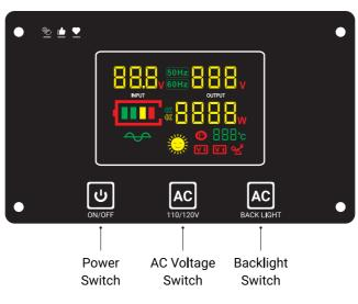
Power Switch: Turns the inverter ON or OFF.
