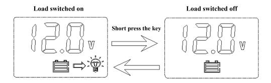
Note: As load start is a type of soft start, display of the load icon on the LCD screen will be delayed after the load is switched on.
